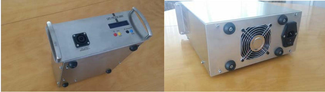
Vertically standing the inverter unit is possible due to the spacer feet on the rear of the unit.
